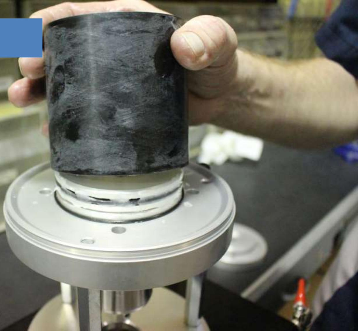
Place even pressure to fully secure the 75-111 cylinder.
