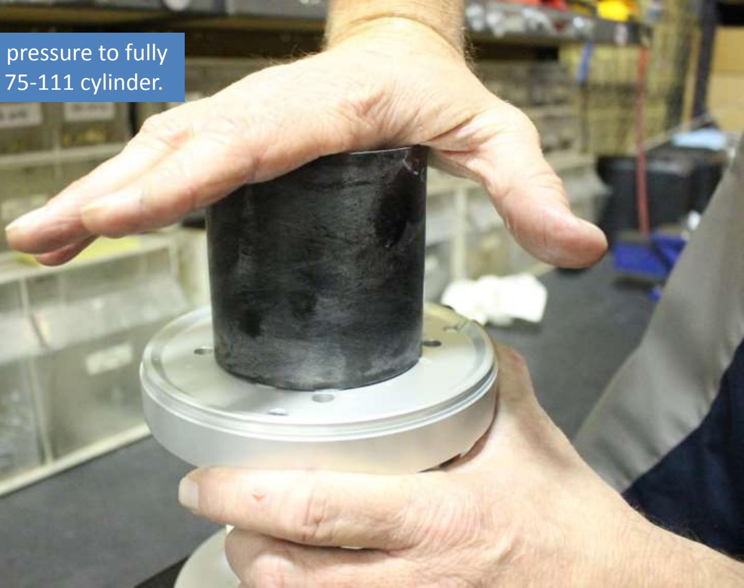
Add 75-125 transfer tube onto the o-ring installed in the 75-113 cylinder head.
