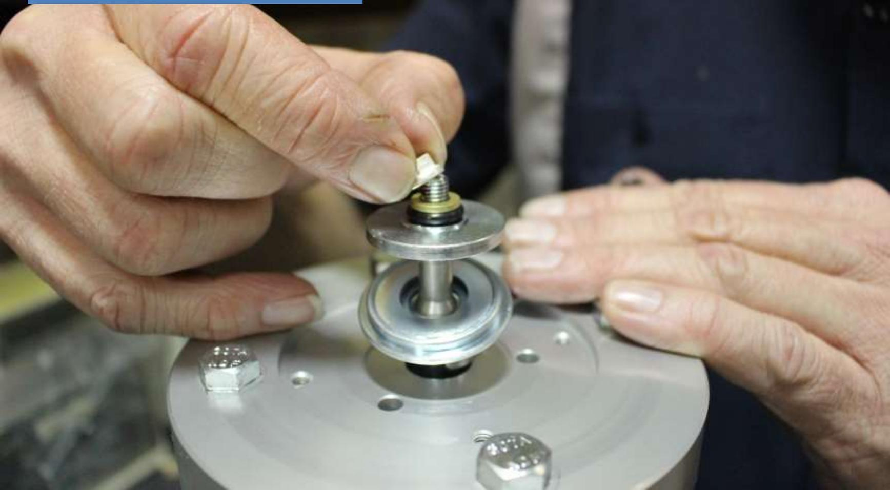
Using the base wrench, hold the trip rod in place to tighten the top locknut.
