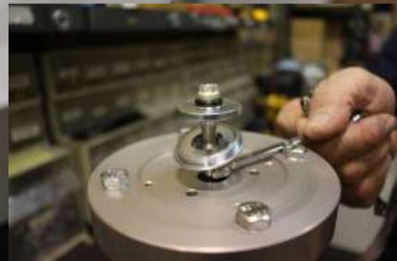
With a pin wrench or screw driver, pull the 75-116 motor rod down.
