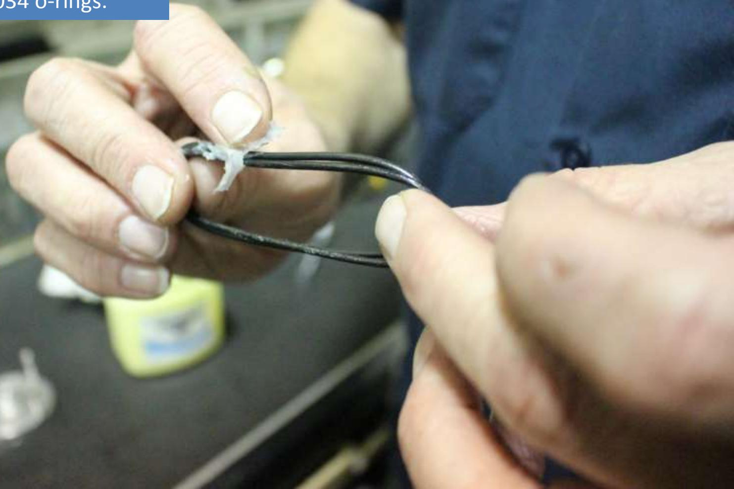
Place 98-7034 o-rings on both sides of 75-129 exhaust spacer.
