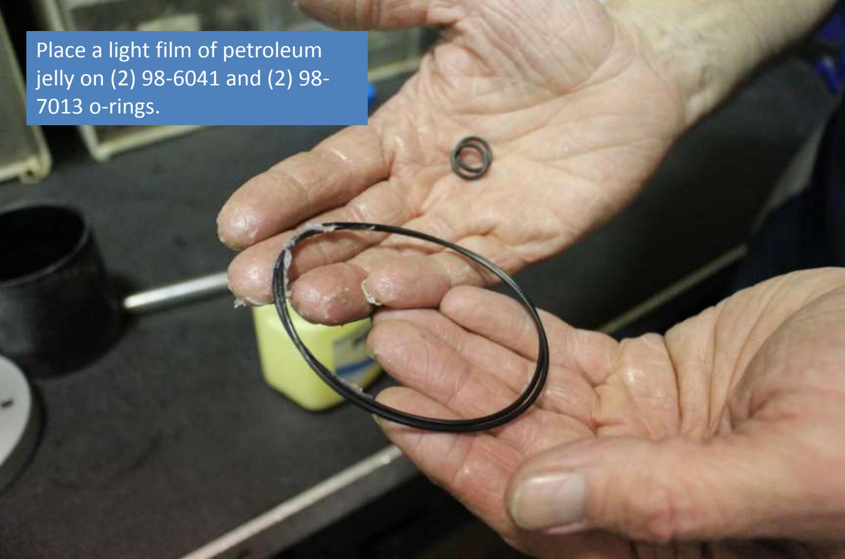
Place the 98-6041 o-ring past the piston and to the cylinder base.
