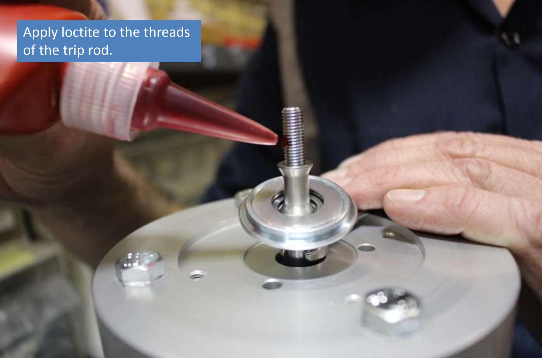
Make sure the 98-6109 o-rings are installed on the 75-161 pole shuttle, and add to the trip rod..
