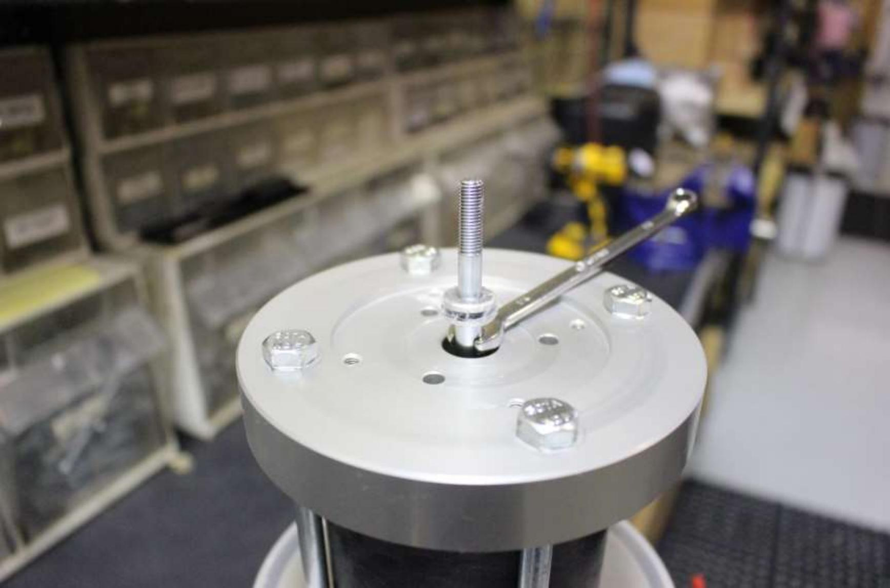
Place the 75-164 spacer on top of the servo piston.
