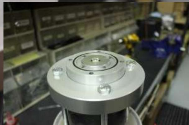
Place 75-115 exhaust cap with the holes facing the left and right of the pump.
