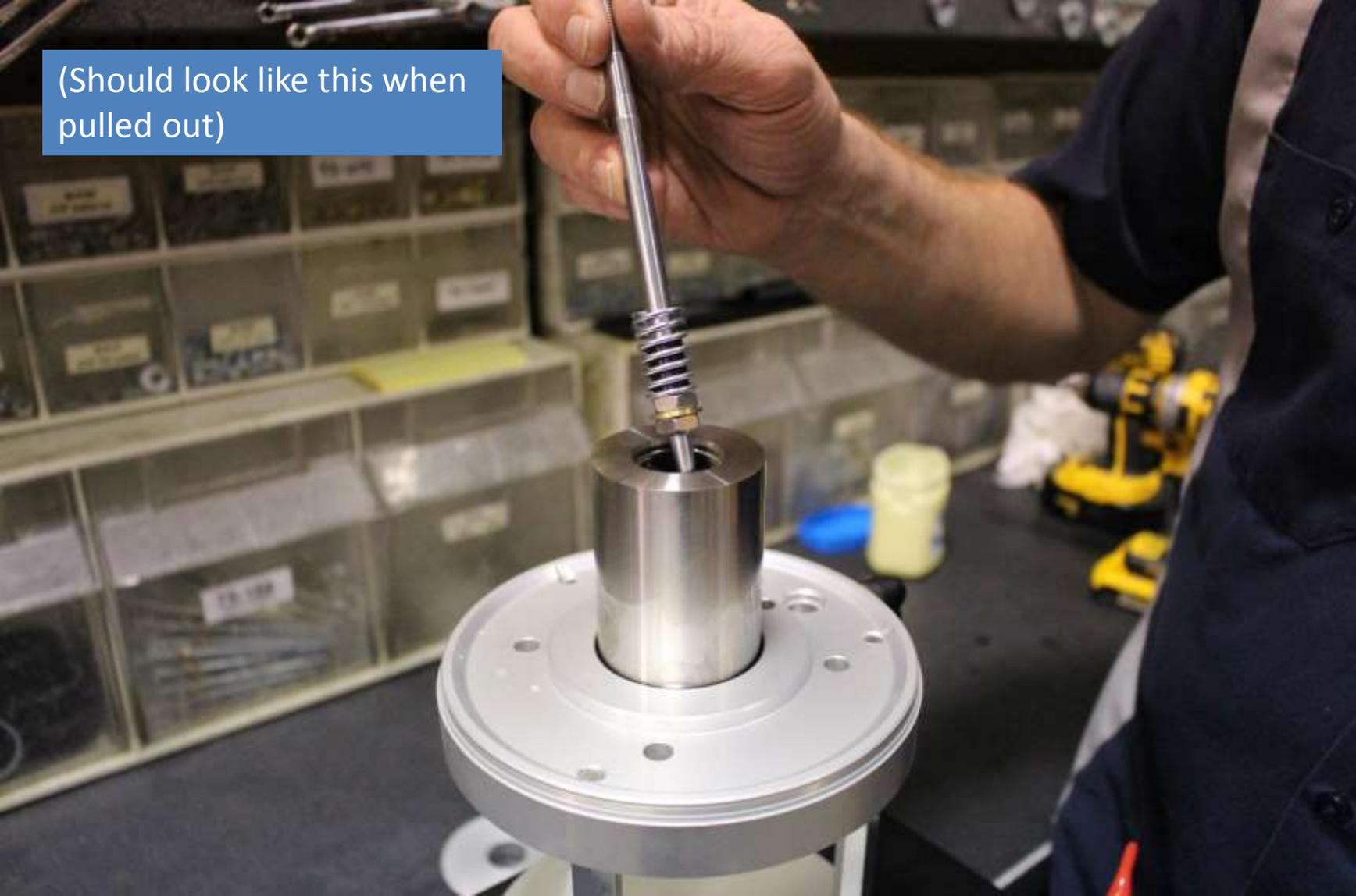
Add 75-114 Piston with center bevel side facing down as shown (98-7234 o-ring should be installed as on the piston).
