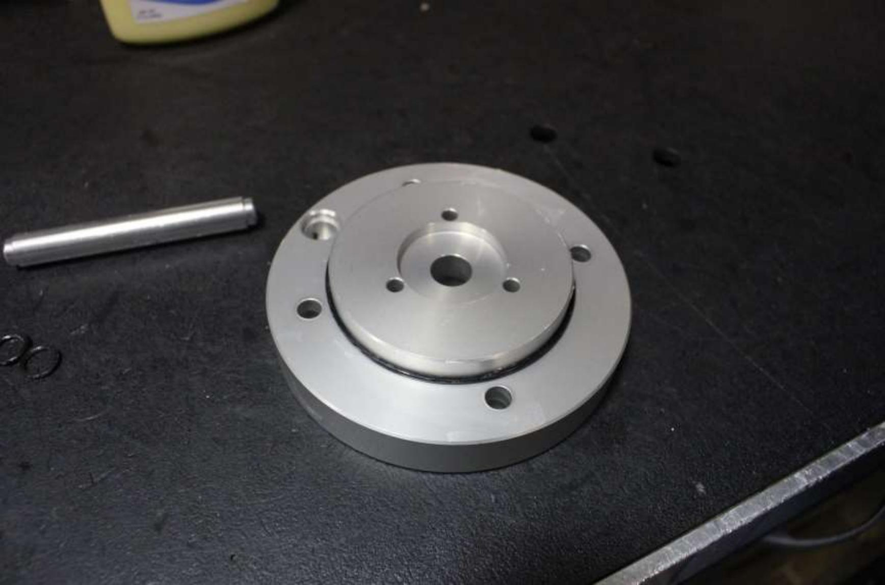
Insert 98-7013 o-ring inside the 75-113 cylinder head cavity as shown.
