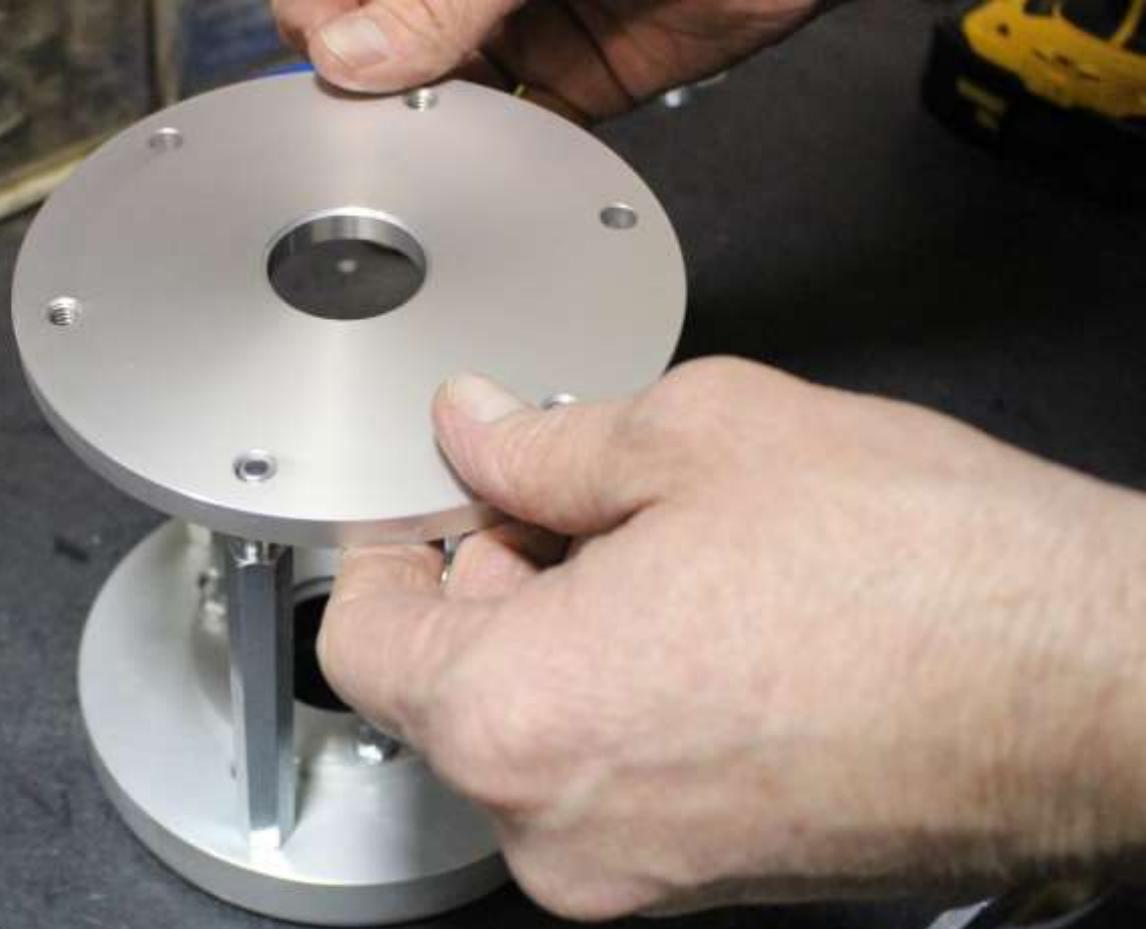
Add lock nuts to ends and tighten to hold in place. You will then flip this over to start assembling the air motor.
