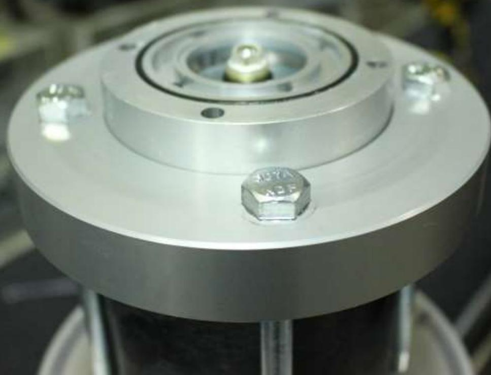
Place second 75-169 magnet assembly over the trip rod as shown. Please note orientation.
