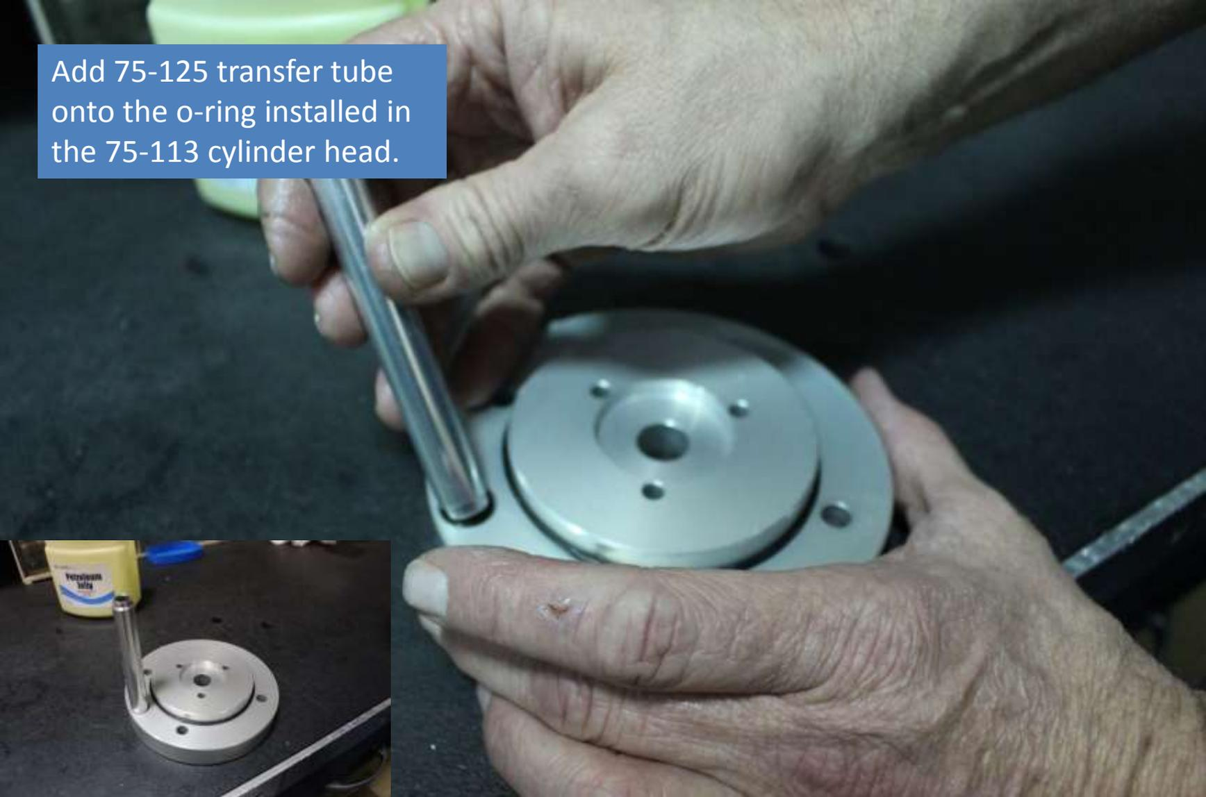
Install the cylinder head with transfer tube as shown.
