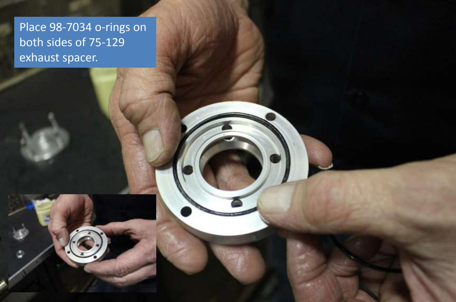
Place 75-129 exhaust spacer on top around the magnet assembly.
