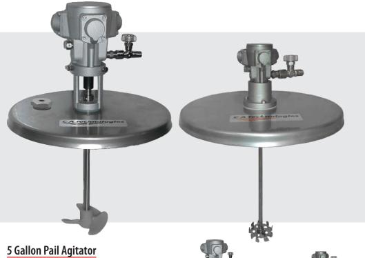
The TechLine economy mixers are for the professional wanting a good mixer at a great price. All of these units are constructed of steel and have stainless steel shafts. The 54-400, 54-410 and 54-450 units have plastic blades, all other models have stainless steel blades. The air motors are piston type motors for longer life.
